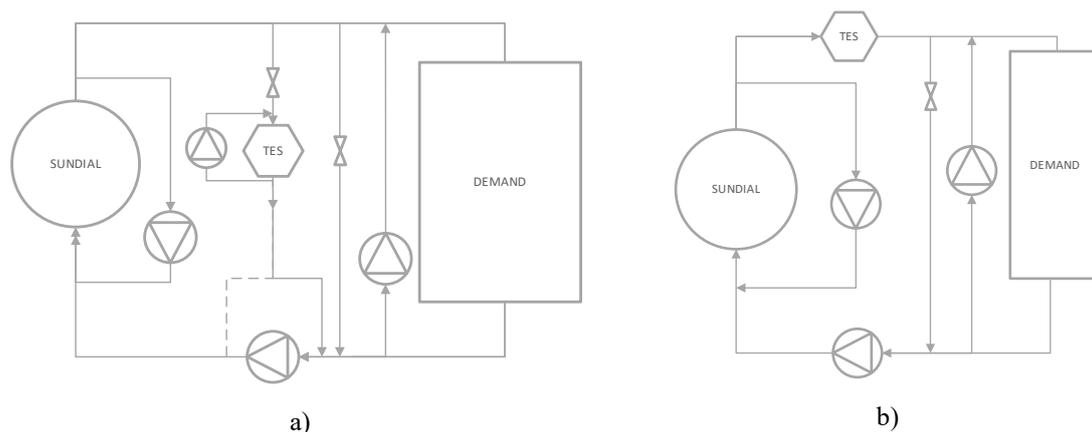
Fig. 1: TES Layouts analyzed: a) SunDial-TES in parallel b) SunDial-TES in series.
