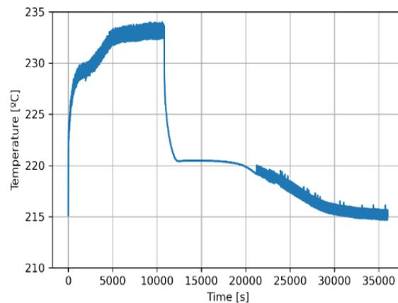
**Fig. 1: Temperature evolution for the charging cycle.**
