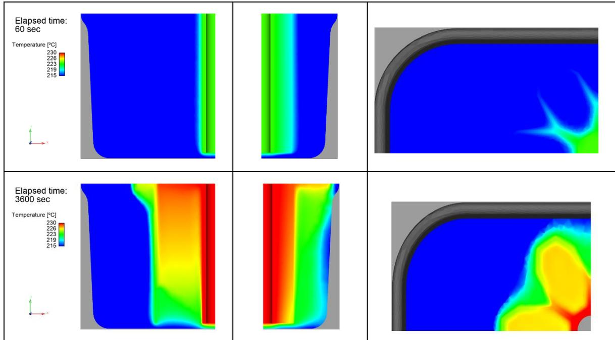
**Fig. 2 Validation case – Temperature**
