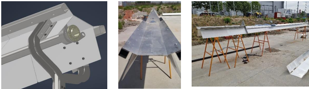
Fig. 5. Detail view of the supporting structure design (left) and receiver assembled next to the SunDial (middle and right)..
