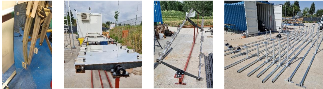
Fig.4. Bent mirror testing the bending-methodology (left), preliminary structures of the mirror lines for high latitudes (middle-left) and low latitudes (middle-right) and final designs ready to be installed (right).
